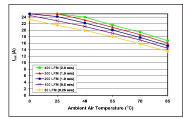
Figure 7: Maximum output power derating curves vs. ambient air temperature for airflow rates of 50 LFM through 400 LFM with air flowing lenghtwise from pin 3 to pin 1 (nominal input voltage).
