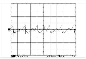
Figure 16: Output voltage ripple at nominal input voltage and rated load current (50mV/div). Load capacitance: one  $1.0\mu F$  ceramic capacitor and one  $10\mu F$  electrolytic capacitor. Bandwidth: 20 MHz. (See Figure 13).
