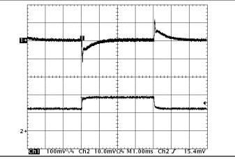
Figure 11: Output voltage response to step-change in load current (50%-75%-50% of Iout(max);  $dI/dt = 0.1A/\mu s$ ). Load cap:  $100\mu F100 \text{ m}\Omega$  ESR tantalum cap and  $1\mu F$  ceramic cap. Ch 1: Vout (100mV/div), Ch 2: Iout (10A/div).
