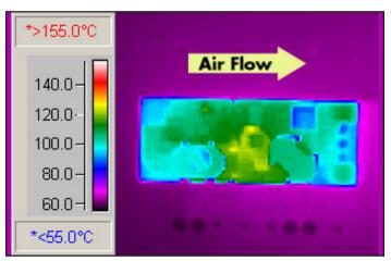
Figure 6: Thermal plot of converter at 21A load current with 55°C air flowing at the rate of 200 LFM. Air is flowing from input to output (nominal input voltage).
