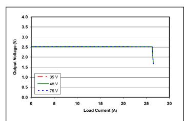
Figure 18: Output voltage vs. load current showing typical current limit curves and converter shutdown points.
