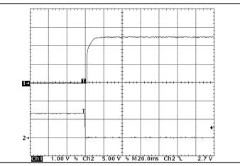
Figure 10: Turn-on transient at zero load (10 ms/div). Ch 1: Vout (1V/div) Ch 2: ON/OFF input (5V/div)
