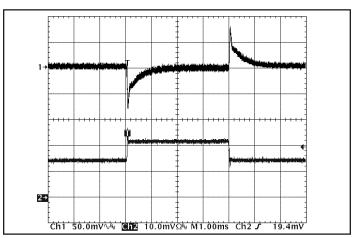
Figure 12: Output voltage response to step-change in load current (50%-75%-50% of lout(max):  $dI/dt = 5A/\mu s$ ). Load cap:  $470\mu F$  30 m $\Omega$  ESR tantalum cap and  $1\mu F$  ceramic cap. Ch 1: Vout (50mV/div), Ch 2: lout (10A/div).
